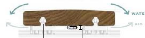
GROOVES are underneath the boards GMM GAP. NO DIRECT CONTACT between the boards and the structure
