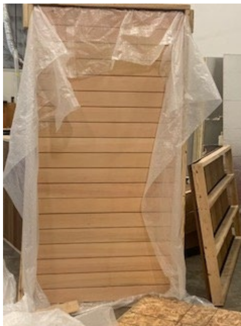
Photo No. 1 Douglas Fir Panel System
